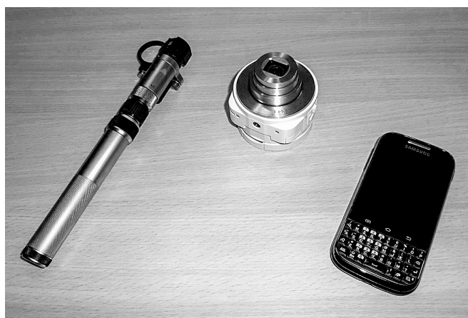
FIGURE 1. Components of our ocular anterior segment imaging system. At left: Heine HSL-150 slit lamp. In the middle: Sony DSC-QX10 lens-styled camera. At right: An Android OS based smartphone
